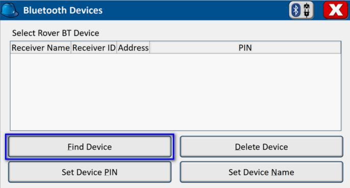
7. Once the desired field gear item has been found (the *Find Device* may need to be run a second time in "noisy" Bluetooth areas), select/highlight the device and tap **Green Check**:
