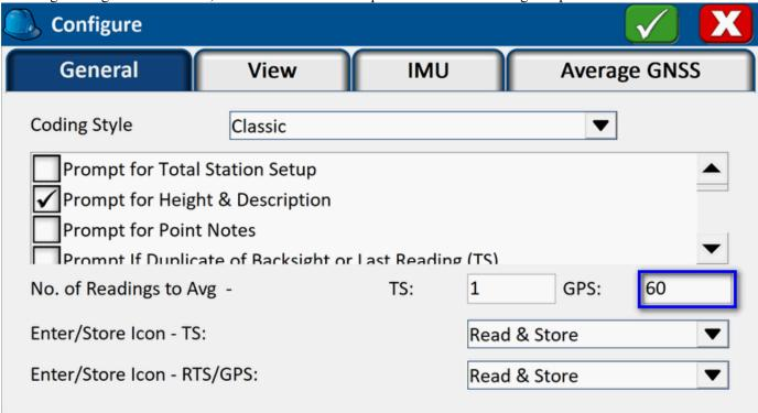
5. (*Optional*) Based on your desired use of correction for tilted-pole, indicate your preferred *IMU* (Inertial Measurement Unit) settings (based on your field equipment):
