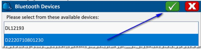
8. The device will be added to the list of desired devices. Select/highlight the device and tap **Bluetooth Connect**: button to pair the controller to the field equipment:
