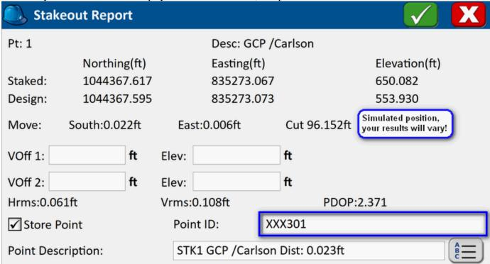
7. Repeat the process by tapping the *Green Arrow* and establishing the next desired point.
