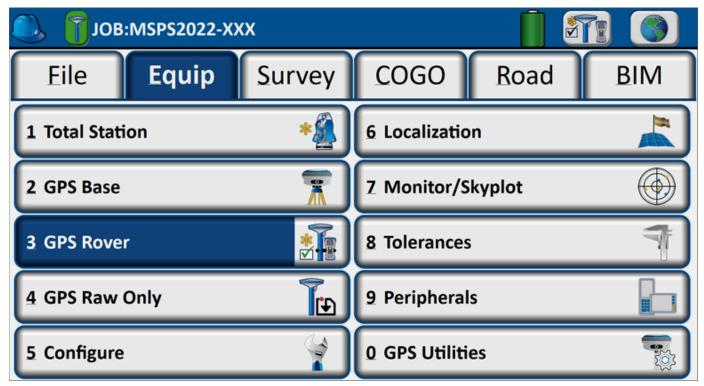
**NOTE**: If working with a traditional base/rover setup, you'll want to first use the **GPS Base** (similar setup instructions as GPS Rover).
