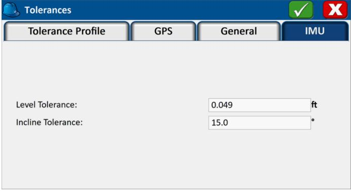
**NOTE**: Upon completion of these desired tolerances, they can be saved into a named **Tolerance Profile** for quick re-use in other similar projects.
