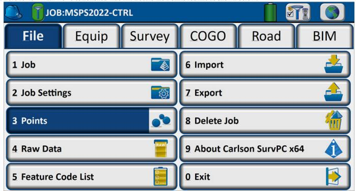
16. Note the different designator(s) of the points. Tap Orange Arrow to dismiss the Points routine.
