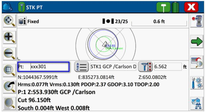
**NOTE**: Make sure to override the default **Point Number** with the pertinent point number syntax as provided for the course. When ready, initiate readings with the "*Store Point*" button (data collector with red dot toward the upper right of the interface).
